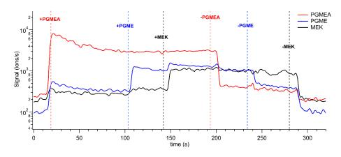
*Figure 2.* Sequential measurement and removal of PGMEA, PGME and MEK demonstrating the detection of these challenging compounds without fragmentation.
