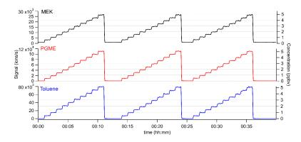
**Figure 4.** To demonstrate reproducibility, accuracy, and time response, three sequences of increasing concentrations of MEK, PGME and Toluene are presented. The left axis shows the measured signal while the right axis shows the measured concentration. The compounds were measured after dilution from a calibration cylinder with a total of 12 compounds, making an overall VOC concentration of ~1200 ppb.
