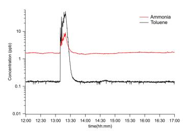
Figure 4. Ammonia and toluene leak detected in an ISO 5 fine chemistry cleanroom.
