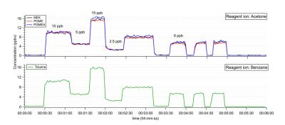
**Figure 1.** Response and recovery time of a ClearFab AMC Monitor. Labels in the plot show target concentrations while the Y-axis shows the measured concentration of selected compounds. The upper plot shows the concentration of MEK, PGME and PGMEA measured with one chemical ionization chemistry, while the lower plot shows the simultaneous measurement of toluene with another chemical ionization channel chemistry.
